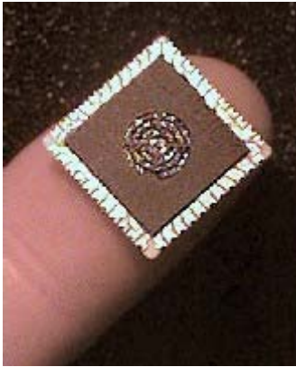
This dime-sized chip can read your unique "light fingerprint." (Photo courtesy of Lumidigm)
